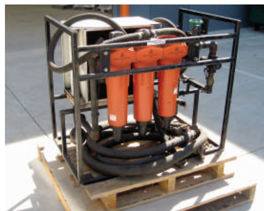
Typical Air Scouring Filter and Cooling Equipment
